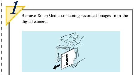
Refer to the instruction manual of the digital camera for the procedure for removing SmartMedia from the digital camera.
